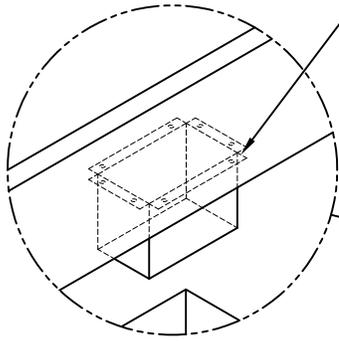
DETERMINE OUTLET LOCATIONS AND FIELD CUT HOLE IN A NEAT WORKMANLIKE MANNER. INSERT ALUMINUM KYNAR OUTLET, FASTEN WITH TWO RIVETS IN EACH FLANGE AND SEAL, WITH NON-CURING SEALANT
