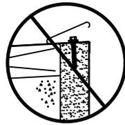
If using an EIFS system, fasten through face w/ fastener of proper length to penetrate through EIFS and attach into structural component
