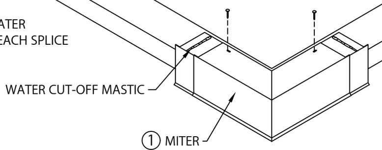
STEP ② POSITION 12'-0" CONTINUOUS CLEAT SECTIONS UNDER SPLICE PLATE AND MITER THEN FASTEN 12" O.C. AS SHOWN WITH PROVIDED FASTENERS. LAP CONTINUOUS CLEAT 1" AT JOINTS.
