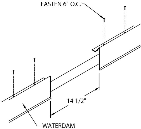
**STEP 1 - WATERDAM / ROOFING MEMBRANE**
