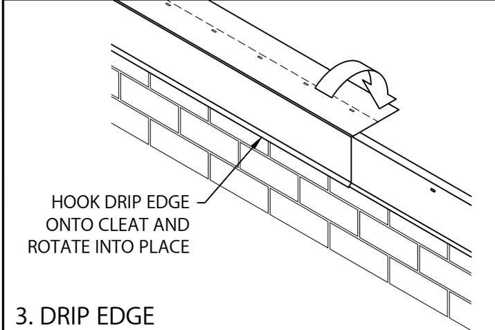
HOOK DRIP EDGE ONTO CLEAT AND ROTATE INTO PLACE
