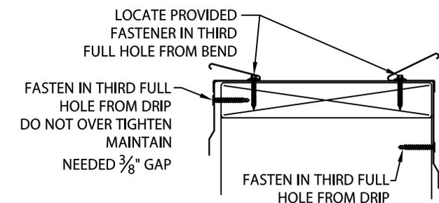
**ANCHOR CLIP FASTENING-DETAIL A**
