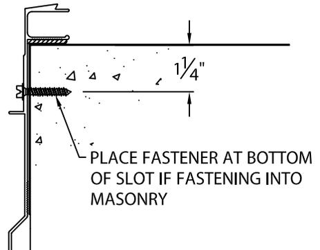
PLACE FASTENER AT BOTTOM OF SLOT IF FASTENING INTO ELIMINAILED-T
