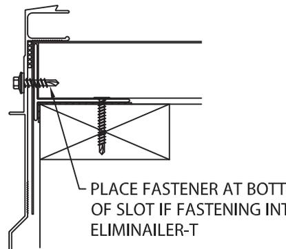
PLACE FASTENER AT BOTTOM OF SLOT IF FASTENING INTO ELIMINAILER-T
