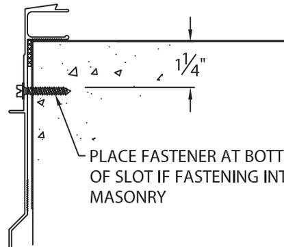
PLACE FASTENER AT BOTTOM OF SLOT IF FASTENING INTO MASONRY
