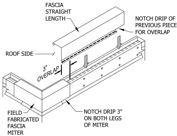
**STEP 2: Installing Fascia Straight Lengths**
