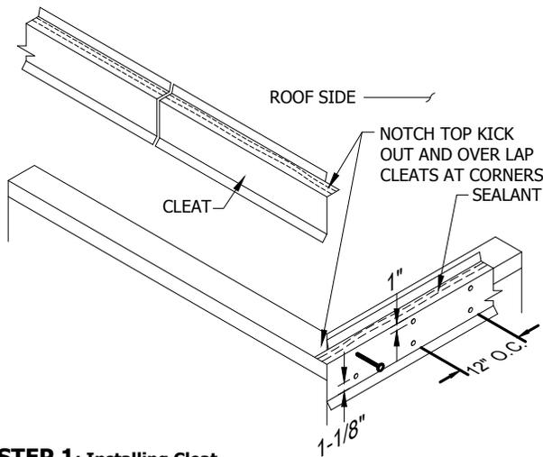
**STEP 1: Installing Cleat**
