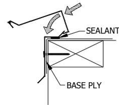
HOOK TOP ONTO CLEAT, ROTATE OVER, THEN PRESS DOWNWARD ON TOP FACE TO SNAP INTO POSITION
