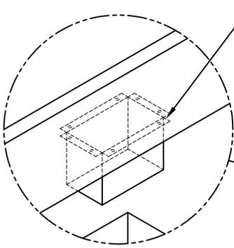
DETERMINE OUTLET LOCATIONS AND FIELD CUT HOLE IN A NEAT WORKMANLIKE MANNER. INSERT ALUMINUM KYNAR OUTLET, FASTEN WITH TWO RIVETS IN EACH FLANGE AND SEAL, WITH NON-CURING SEALANT
