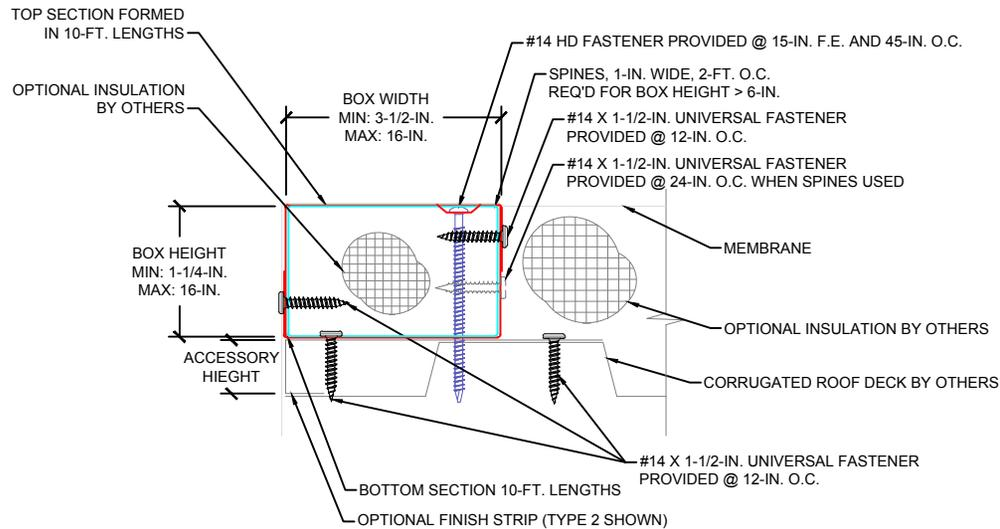
PRE-DRILL WITH 3/16-IN. DRILL BIT FOR MASONRY CONDITIONS.
