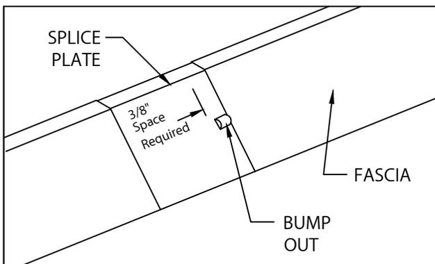
5. INSTALL 12'-0" FASCIA COVER SECTIONS. INSERT ONE SPLICE PLATE UNDER EACH OF THE FASCIA COVERS. INSTALL COVER BY PUSHING DOWNWARD UNTIL FASCIA COVER IS ENGAGED TO WATER DAM ALONG ENTIRE LENGTH. CONTINUE TO INSTALL FASCIA COVERS, FIELD CUTTING WHERE NECESSARY USING FINE TOOTH HACKSAW.
