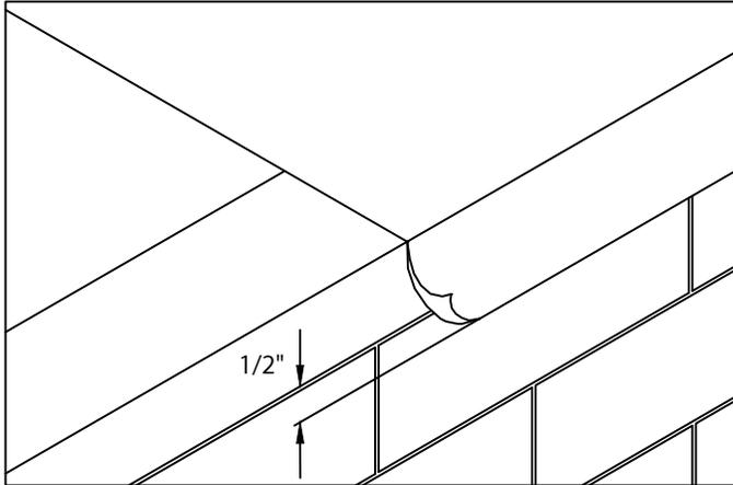
1. POSITION MEMBRANE OVER THE ROOF EDGE AND DOWN OUTSIDE FACE OF WALL, COVERING TREATED WOOD NAILER(S) COMPLETELY. ALLOW  $\frac{1}{2}$ " EXCESS MEMBRANE.
